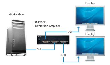
The Emerge DA1200D DVI-D distribution amplifier provides transparent distribution of signals to two display devices using DVI cables. Fully HDCP complaint, the distribution amplifier inhibits the unauthorized distribution of digital video material through copying
