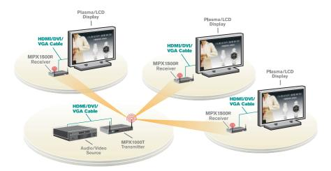
The Emerge MPX multipoint extender solution includes a transmitter and receivers for wired or wireless professional audio-visual applications. Interchangeable modules are available for MPX1000T input of analog VGA signals or digital HDMI/DVI signals. The MPX1500R receiver features a universal media input port based upon a DVI-I dual-link connector.
